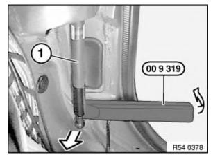
Pry out gas spring strut (1) at bottom with special tool 00 9 319 and remove from the vehicle.
